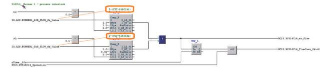
• In case of rarely used PC elements, which are not defined in conversion tool yet, they are replaced by red **placeholders**. At the same time all input / output logic connections are translated and maintained. Names of placeholders are added to the FunctionBlocks definition tab. Just new FB definition in User Lib remains to be done manually.
