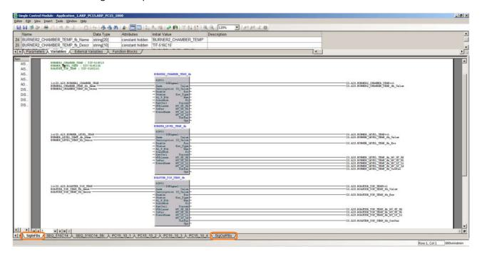
RealIO and BoolIO variables are created locally in the same SCM along with corresponding IO function block in case of Local preference, or globally in case of global preference. IO variables are furnished with original IO name, Range, Unit and Fraction in variable description.
